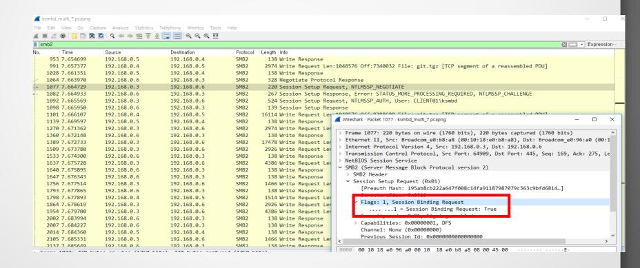
Client sending interleaved write requests to dual channels (192.168.0.3, 192.168.0.4)
